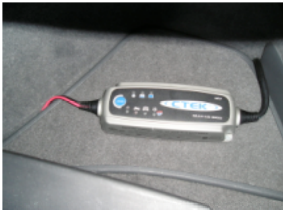
Fig. 2. Positioning of trickle charger in rear luggage compartment of PHEV.
