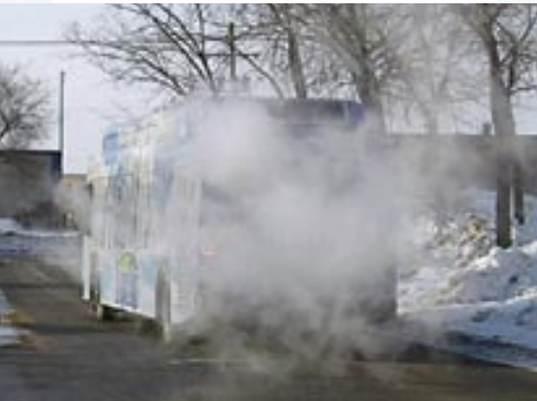
The water vapour exhaust from the bus was clearly visible in cold weather.
