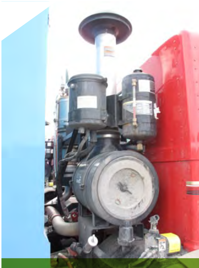
Figure 11 - EBI Conventional Air Intake System
