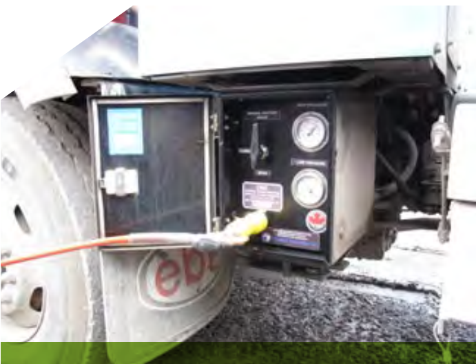
Figure 19 - Fuel Gauges Below EBI Truck Tank Enclosure
