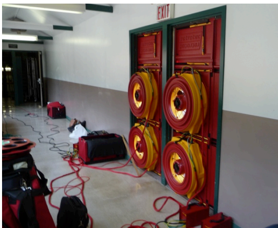
Figure 1 – Multi-Fan Blower Door System Used for Airtightness Testing
